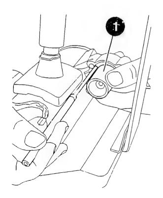
Disassembling bearing-end plate
